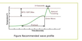
The upper side temperature of the board should not exceed +150°C.
